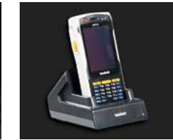
PDA Programmer Wireless two-way communication using a Windows based PDA with infra red port. Flash code, range and photocell switch level etc. can be set. The Programmer can also retrieve the event log.
