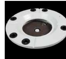
Installation The bottom plate supports installation on structures using 3 x M12 bolts or 4 x M12 bolts on a 200mm diameter.
